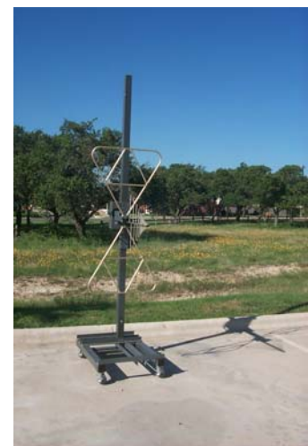
6. Antenna mounted on mast in vertical polarization.
