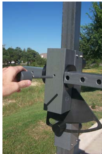
2. Remove polarization locking pin.
