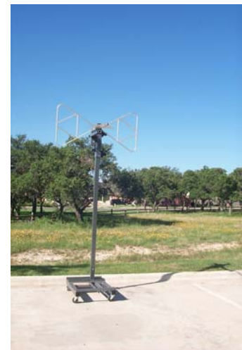
6. The antenna mounted on the mast in a 3m position.
