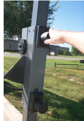
2. The positioning gimbal secures the mounting arm to the mast.
