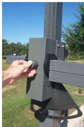
5. Replace polarization locking pin.
