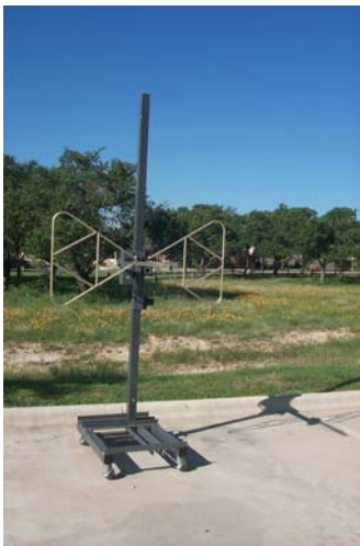
1. Antenna mounted on mast in horizontal polarization.
