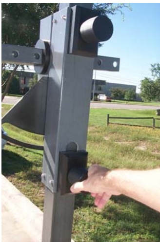
4. Support the mounting arm and loosen the lower vertical positioning screw. The mounting arm is released.
